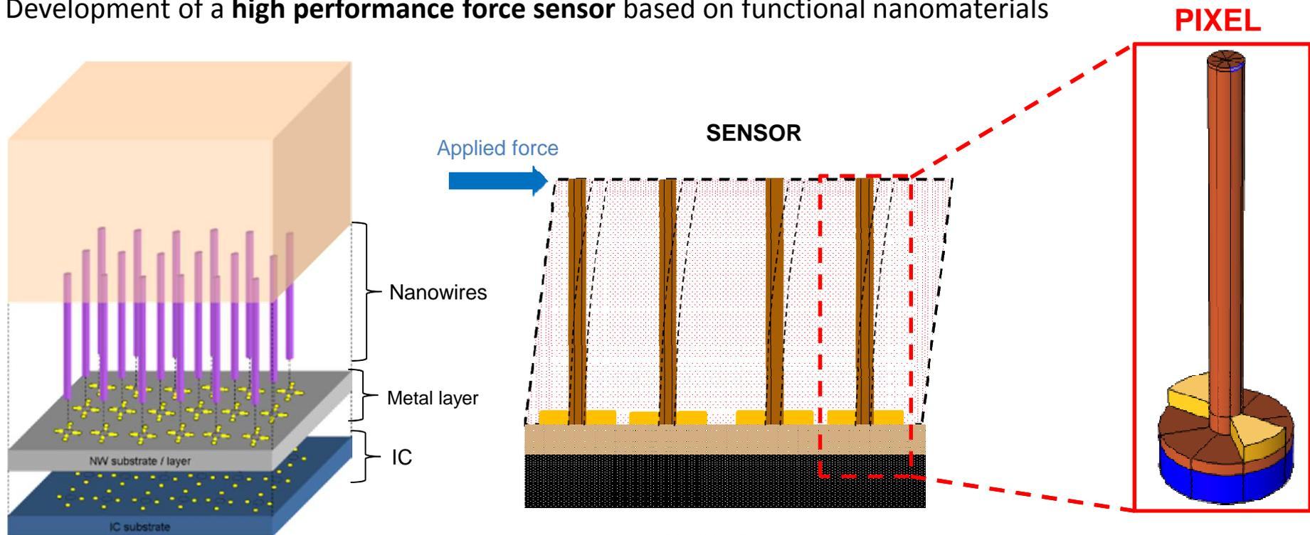
Piezoelectric response impacted by nanowires characteristics (Hinchet et al., IEDM 2012)
