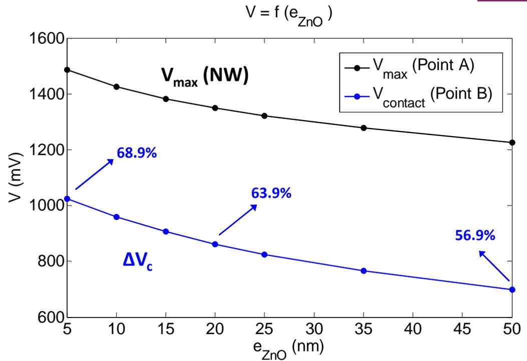
Collection efficiency =  $\Delta V_c / V_{max}$
