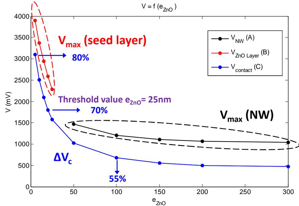
$$\text{Collection efficiency} = \Delta V_c / V_{max}$$
