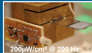
Piezoelectric AlN harvester
