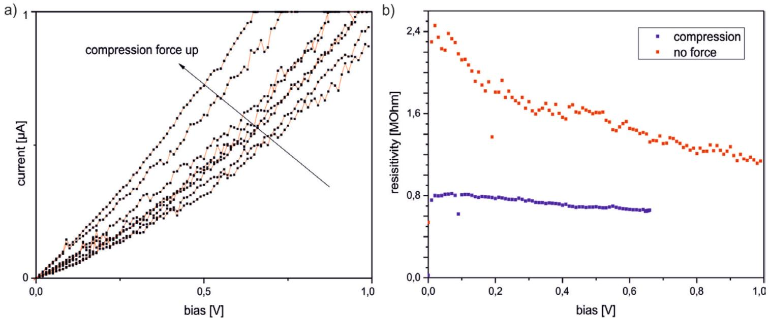
ZnO is “piezo-tronic” material -> resistance is a function of applied force!
