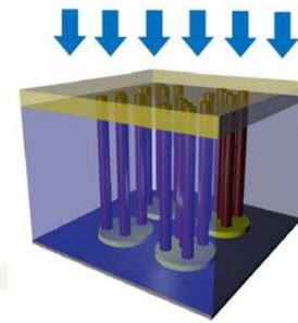
Multi-NW pixel embedded into polymer matrix
